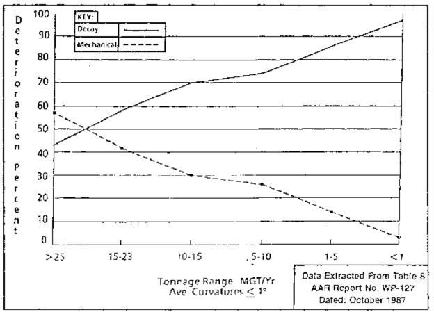
Figure 1 - Causes of tie failure
