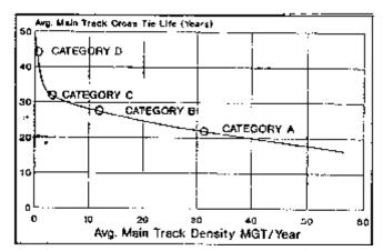
Figure 2 - Tie life versus tonnage, from 1978 industry statistics<sup>2</sup>
