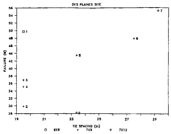
Figure 2 - Failure rate vs. tie spacing
