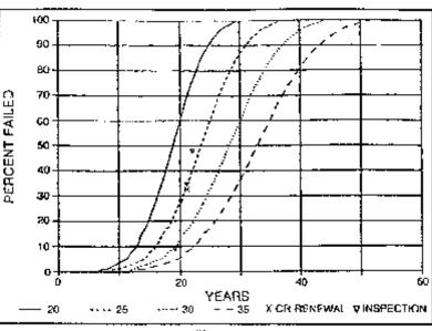
Figure 3 - Forest products curve for various average life values: Cumulative failures versus years in track, at mile 266'
